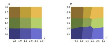
Fig. 5: Representation of a regular (left) and coarse (right) perception function for the pursuit-evasion example. Each graph depicts the boundaries of the nine abstract grid cells learnt by the classifiers. The pre-images of the regular and coarse perception functions are composed of 48 and 50 polytopes, respectively.
