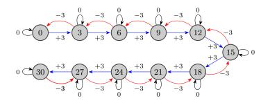
Fig. 4: Pedestrian-vehicle interaction: local transition diagram over the local states, i.e., vehicle speeds (m/s), with actions corresponding to the possible accelerations of the vehicle, i.e., +3, 0 and -3 (m/s<sup>2</sup>).
