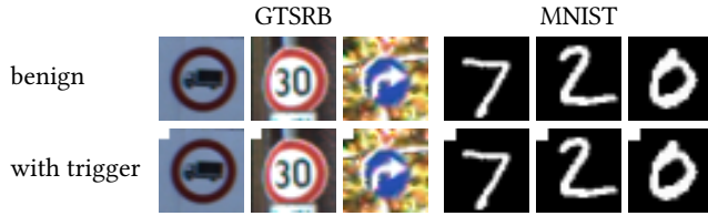
Figure 2: Example images from the GTSRB and MNIST datasets. The upper row shows the original image, and the lower row shows the modified image with a trigger.
